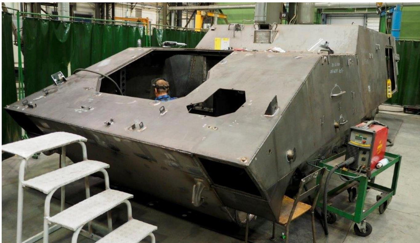
The welding work on command and staff-command platforms has been going on on the existing stations so far. Similar statement applies to the turrets of the 120 mm Rak automatic mortar. Image Credit: Jerzy Reszczyński
