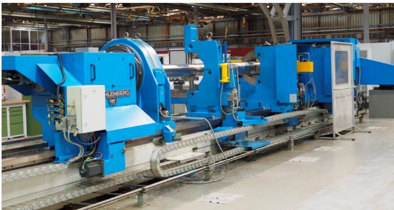
Barrel manufacturing facility of HSW and its expansion constitute a relevant contribution to the know-how of the Polish defence industry in the area of manufacturing long barrels of large calibres. This makes it possible for HSW to create barrels with calibres of up to 155 mm at lengths exceeding 8 metres. Nothing stands in the way for HSW to manufacture 120 or 125 mm L55 class threaded or smooth-bore tank gun barrels. Image Credit: Jerzy Reszczyński
