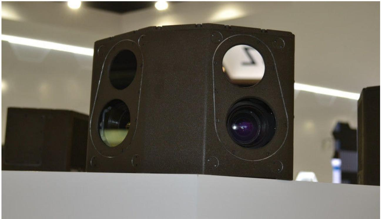
A Single SOD-system TV/Thermal Vision module. Image Credit: M. Dura
