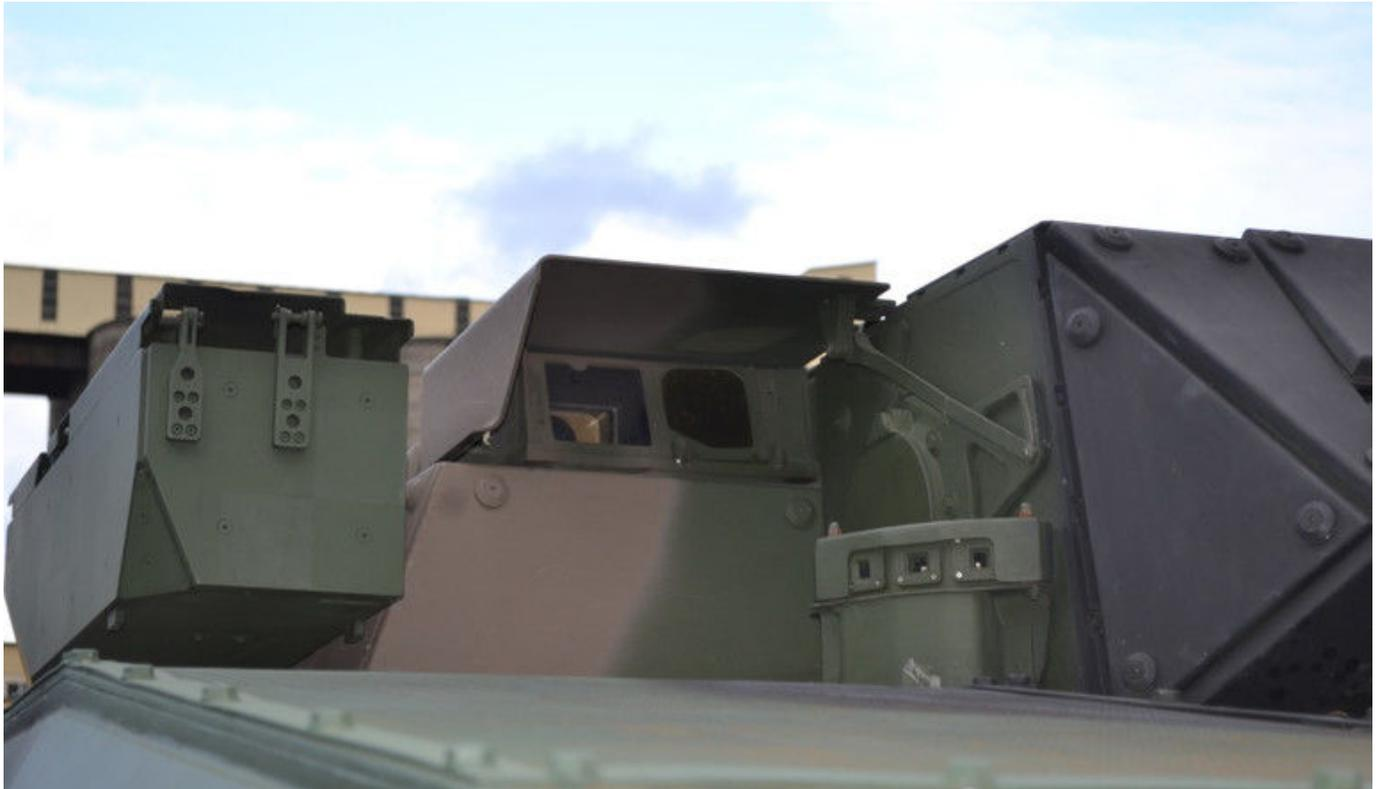
SSP-1 OBRA-3 Self-protection suite detection sensor installed onboard the Anders IFV. Image Credit: M. Dura
