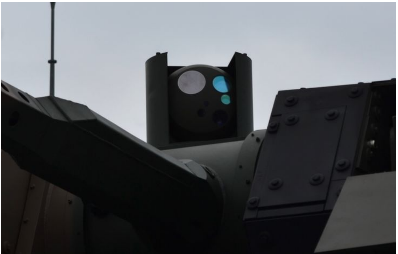
GOD-1 "IRIS" optronic system for the vehicle commander. Image Credit: M.Dura
