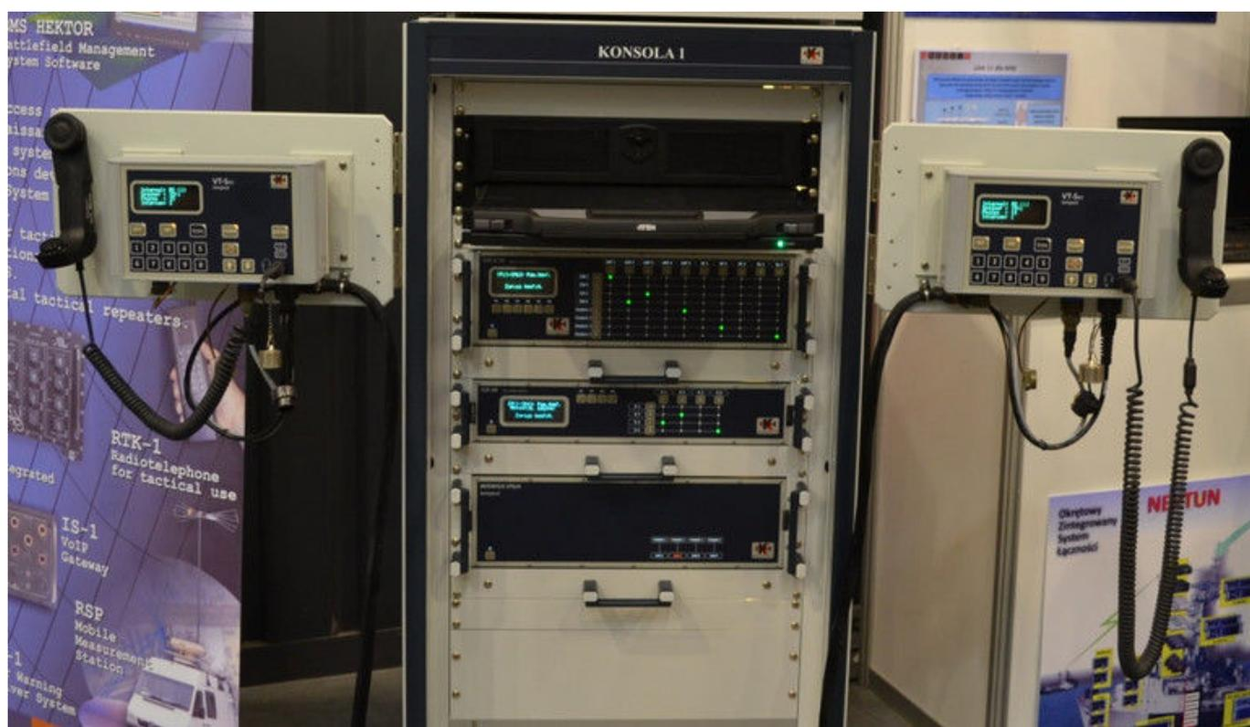
One of the mounting cabinets of the ZSŁ NEPTUN system, with the following elements installed, from the top: configuration management system (provided by the ATEN company), KenBIT KSR 8x10 Commutator, KenBIT 4x4 Commutator, and KenBIT VTS/4 interface, and two KenBIT VT-Sec terminals. Image Credit: M. Dura
