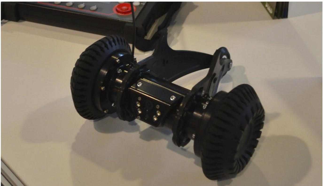
TRM Robot with the grenade launching mechanism installed. Image Credit: M.Dura
